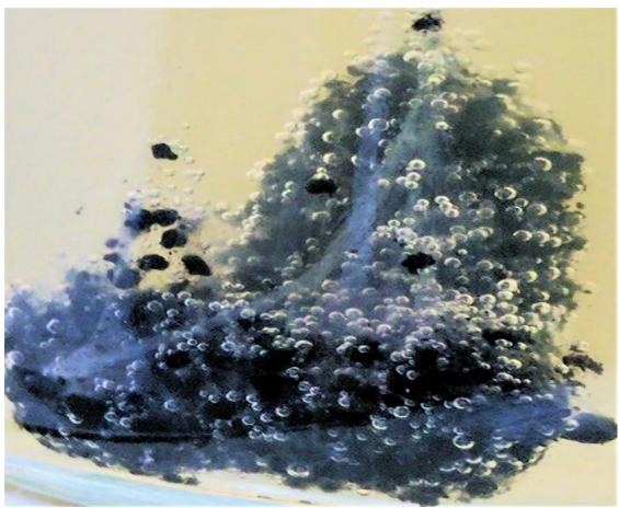
Biofilm formation in several of the test bottles was so extensive that the grains of carbon or the char were completely surrounded by goo and liquid in the bottle had the viscosity of egg-drop soup.
