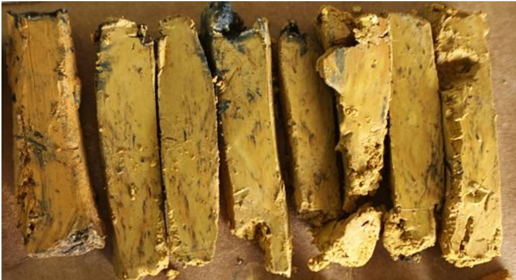
This is a picture of 2.25-inch direct push cores sliced vertically. The black inclusions are BOS 200®. It is visually evident that the BOS 200 has distributed well using high energy, high flow techniques.
