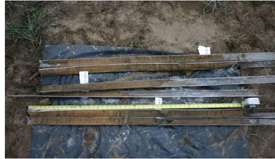
FIGURE 10. Evidence (black striping) of thorough BOS 100 ® distribution.
