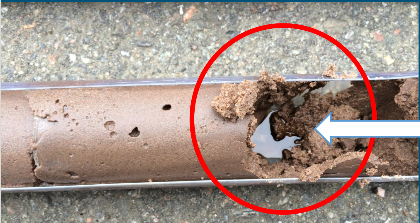
DNAPL evidence MW27 soil core
